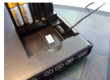
Detail of battery case for reloadable batteries with integrated solar panel socket.
